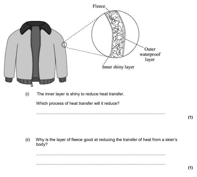
(b) A student tested four different types of fleece, J, K, L and M, to find which would make the warmest jacket. Each type of fleece was wrapped around a can which was then filled with hot water. The temperature of the water was taken every two minutes for 20 minutes.
