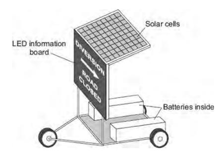
The batteries power the LEDs used in the information board. The solar cells keep the batteries charged.
