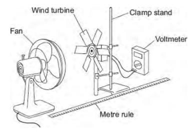
The fan was used to turn the wind turbine.
